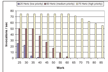
Figure 30: Effect of Increasing Workload in Real-time CORBA without Lanes: Server Thread Pool Priority = High
