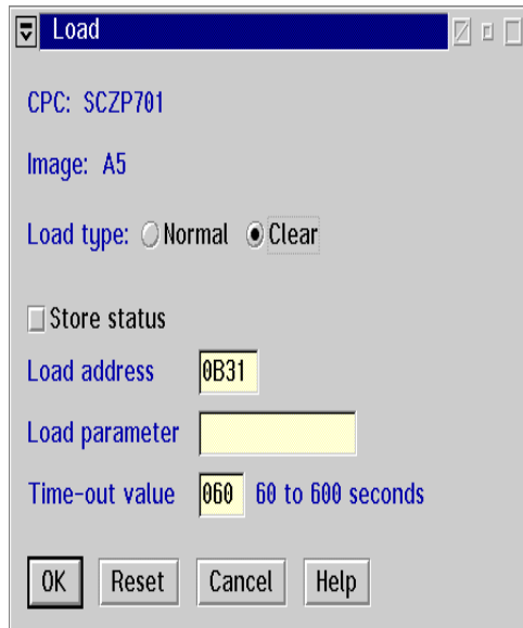
Figure 14. Load with unit address of tape drive
